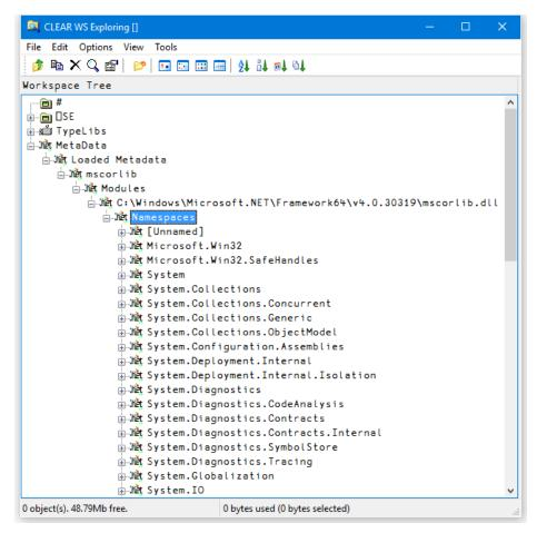
Opening the *System/ Classes* sub-folder causes the Explorer to display the list of classes contained in the .NET Namespace *System* as shown in the picture below.
